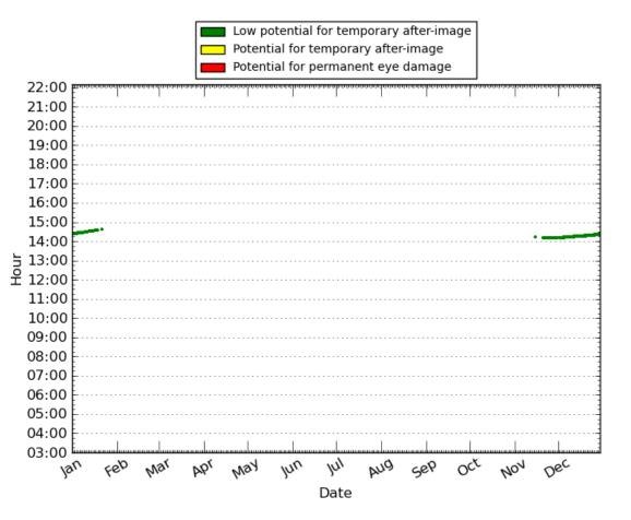
Predicted glare and potential ocular hazard from observation point 5 (3 km from touchdown) on approach to Runway 24. A low potential for ocular impact is predicted.
