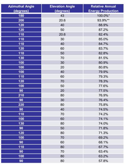
Alternative PV array configurations that are predicted to produce no glare to the ATCT (unless otherwise noted).
