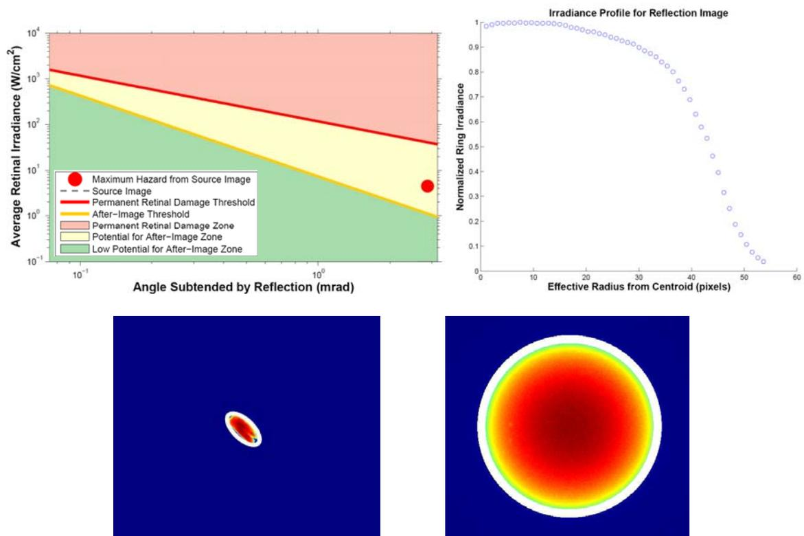
Figure 6. Output from web-based glare evaluation: hazard analysis of dish glare located 29 m from observer (top left), normalized irradiance profile of reflected image (top right), normalized flux map of reflected image (bottom left), and normalized flux map of sun image (bottom right).
