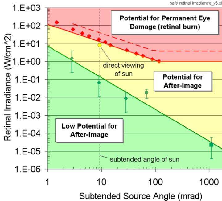
**Figure 2. Safety metrics and potential impact of viewing glint and glare as a function of retinal irradiance and subtended source angle (from [2]).**
