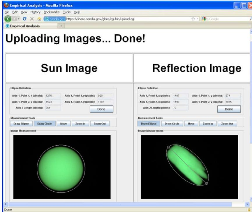
Figure 5. Images of the sun and reflection (glare) taken using RAW image format. The user selects drawing tools (circle, ellipse, zoom, move) to outline relevant portions for processing.
