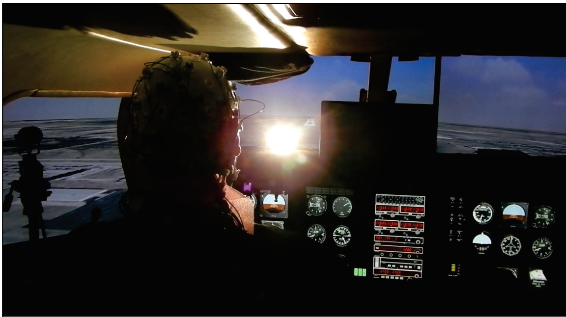
Figure 2. Interior view of the AGARS cockpit, with the 0-deg GLD triggered.
