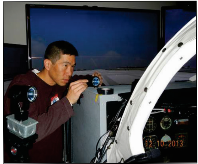
Figure 1. Placement of two of the Glare Simulation Devices are at 5 deg and 50 deg.
